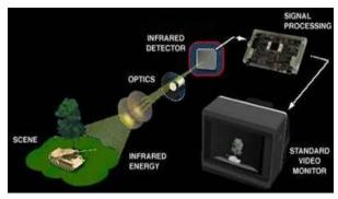
Thermal imaging working is base on light. The amount of energy in a light wave is related to its wavelength: Shorter wavelengths have higher energy.
